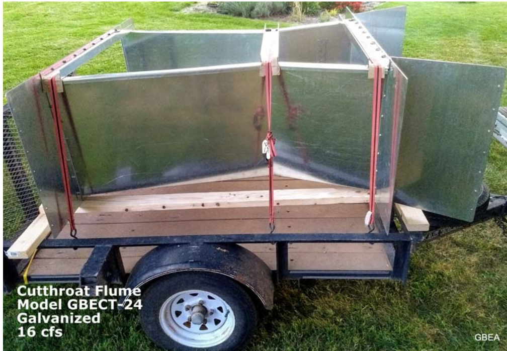
Photos 8. Cutthroat flume, Model GBECT-24. A 24 inch throat with a max cfs of 16.0 cfs. Galvanized steel model, 12 gauge.
