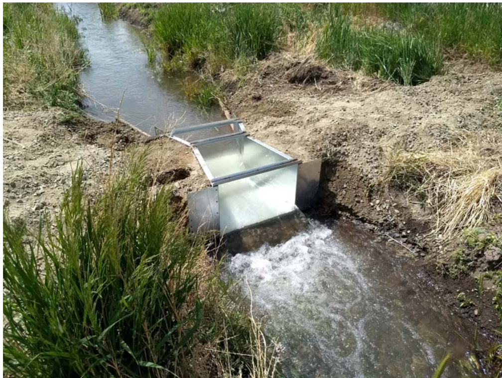
Photos 3 and 4. Cutthroat flume, Model GBECT-16. A 16 inch throat with a max cfs of 6.0 cfs., flowing at 2 cfs. Galvanized steel model, 14 gauge. This is a free flow conditions.
