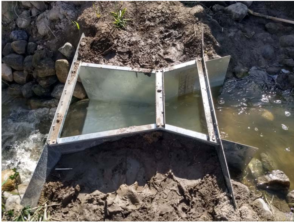
Photos 7. Cutthroat flume, Model GBECT-16. A 16 inch throat with a max cfs of 6.0 cfs., flowing at 1.0 cfs. Galvanized steel model. 14 gauge. This is a free flow conditions.
