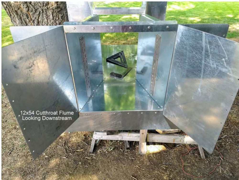
Photos 5 and 6. Cutthroat flume, Model GBECT-12. A 12 inch throat with a max cfs of 8.0 cfs., flowing at 4.97 cfs. Galvanized steel model. 12 gauge. This is a free flow conditions. Bottom photo is during assembly.
