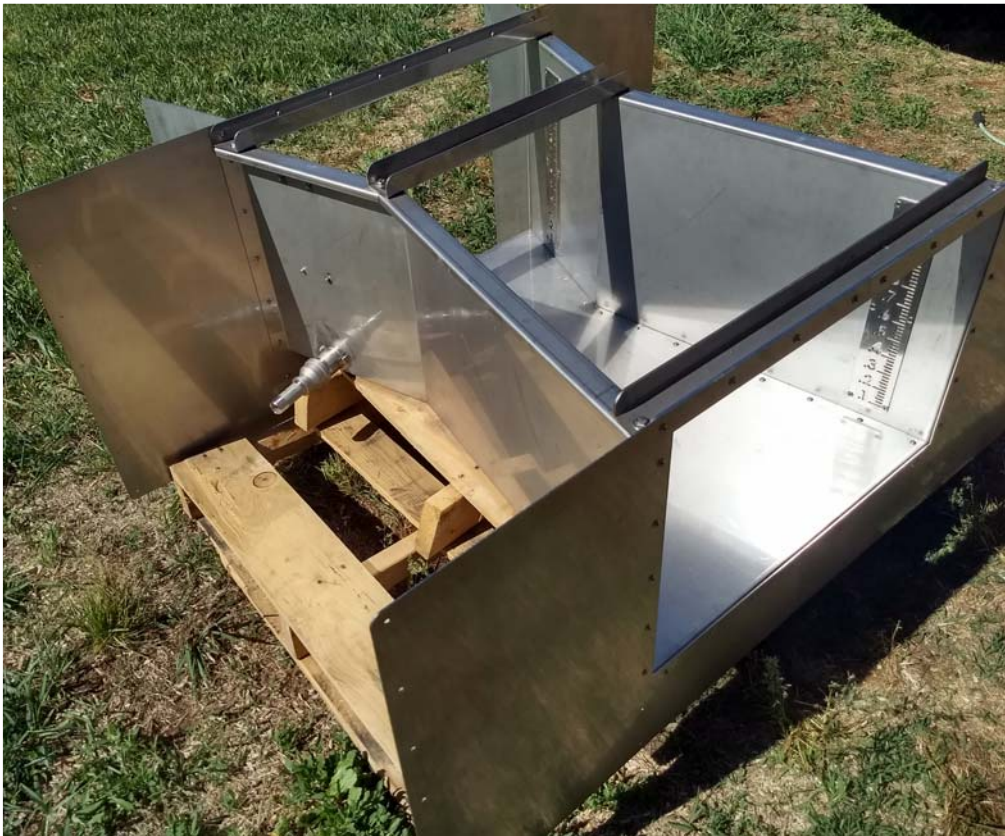
Photos 1 and 2. Cutthroat flume, Model GBECT-16s. A 16 inch throat with a max cfs of 6.0 cfs. Stainless steel model. Top photo inlet, bottom outlet.
